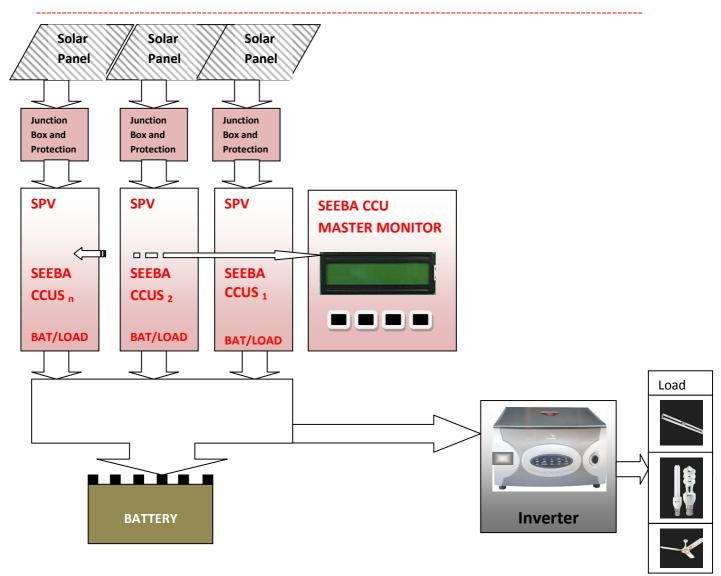
Typical Connection Diagram Showing "n" CCU s Monitored and Controlled by Master Monitor.
